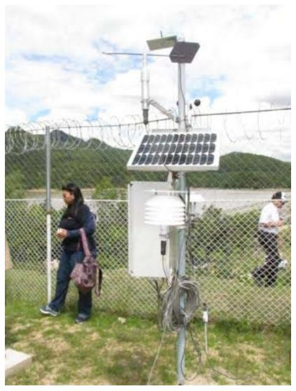
Photo 3: One of the 46 weather monitoring stations installed around Tegucigalpa
